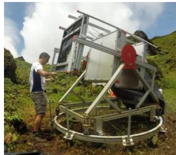
Fig. 2 – Muon telescope in operation on La Soufrière in July 2015. The telescope is remotely controllable.
